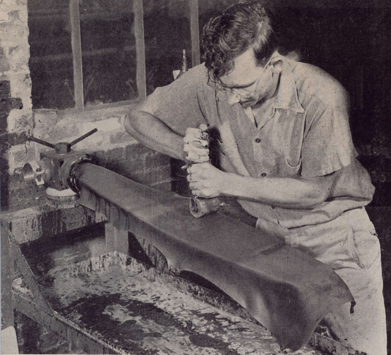
5—The plastic sheet is hand rolled to the blade for the purpose of eradicating irregularities and achieving bond
