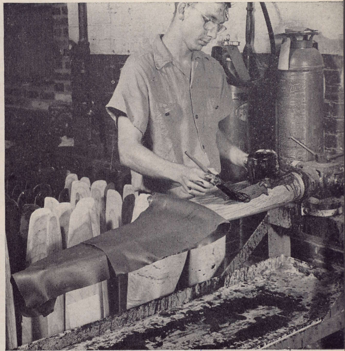
3—(Left) After suspension for an hour in a softening solution the nitrate sheet is ready for application to the blade. 4—(Right) Plastic cement is first applied to top side of blade and to half of plastic sheet
