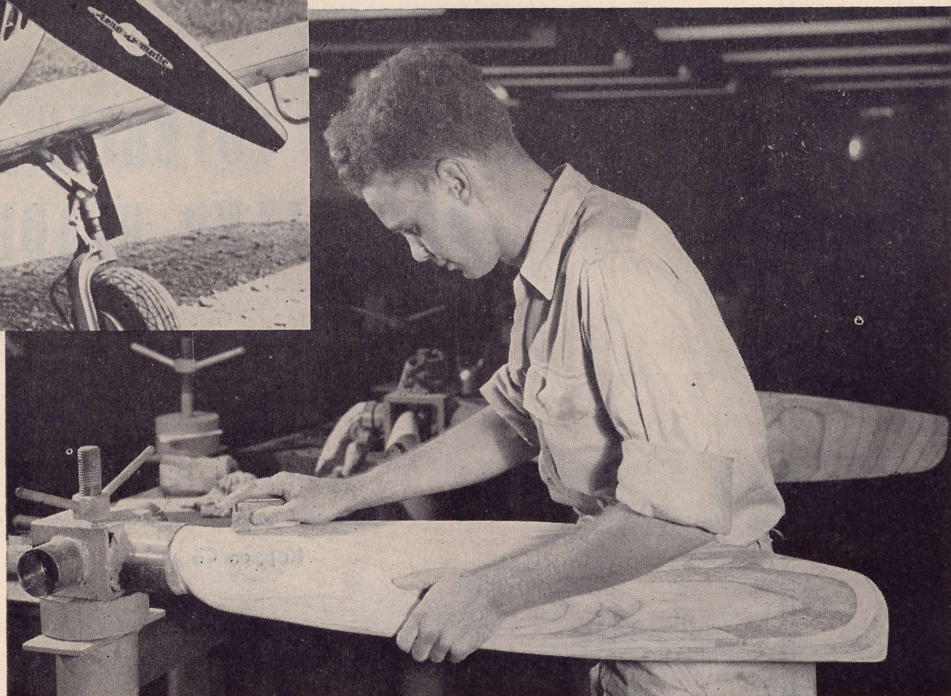
2—A light sanding of wood blade is performed locally to bring the blade to an accurate template fit. The blade is carved from laminated maple veneers
