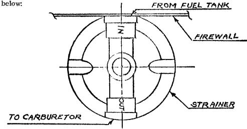
If the fuel strainer is not installed as indicated above, it should be reversed for proper fuel flow.
