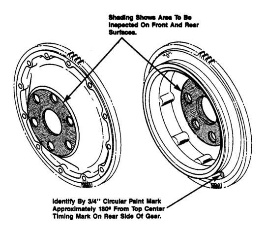
Figure 1. Starter Ring Gear Inspection Areas
